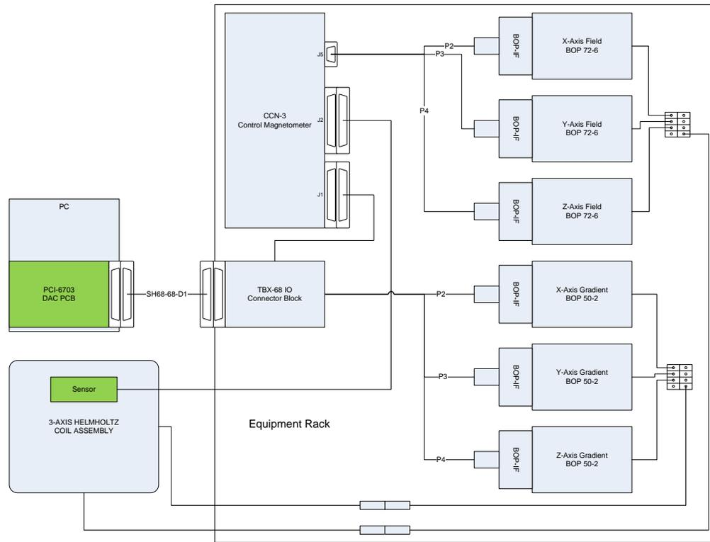
**Figure 4-1 Block diagram of HCS01CL with Gradient three-axis Helmholtz coil system.**
