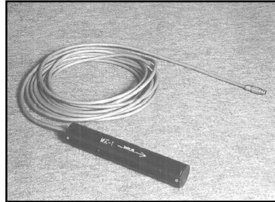
The **MGC-1A** also includes a calibration winding that can be used to verify performance or perform a health check.
